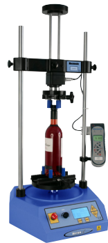
Closure torque test
