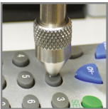
Keypad compression test
