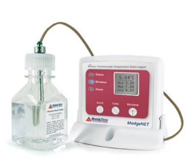
The thermocouple probe is detachable from the data logger
